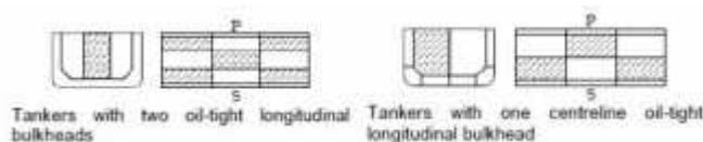
Fig 1.3.1 "Stagger test" – checker board pattern
