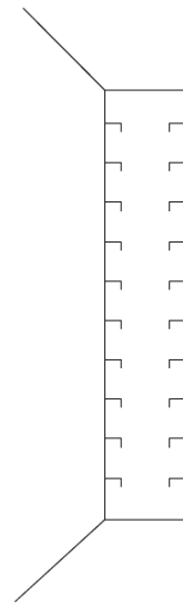
Ordinary longitudinal structure in double skin tank
